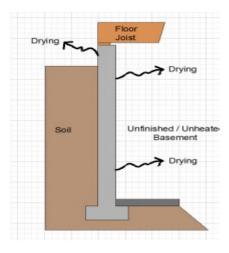
Depending on the time of year it's possible that all that humidity in the air will turn around and condensate on the cool concrete surface if the dew point is correct. The point here though is how moisture in the form of water vapor leaves the foundation walls and migrates into the basement space or outside above grade.
